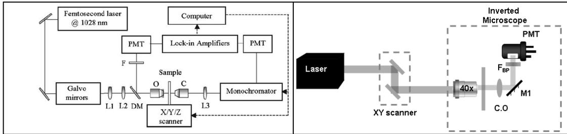
Fig. 1. Schematic representations of both THG setups. Left panel shows the experimental set-up for 1028nm PMT: photomultiplier tube, DM: dichroic mirror, O: objective, C: condenser, F: filter and L1/L2: telescope. Right panel shows the experimental set-up for 1550nm. Laser is the FemtoFiber FFS laser, C.O is the condenser optics; M1 is a silver mirror; FBP is the set of band pass filters (transmittance = 512 – 521nm); and PMT is the photo multiplier tube.
